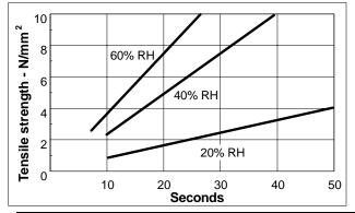
Where cure speed is inadequate, due to low relative humidity, or large gaps, a LOCTITE ACTIVATOR may be used. This can, however, lead to a reduction in eventual strength of the bond and careful testing is recommended before use in production.
